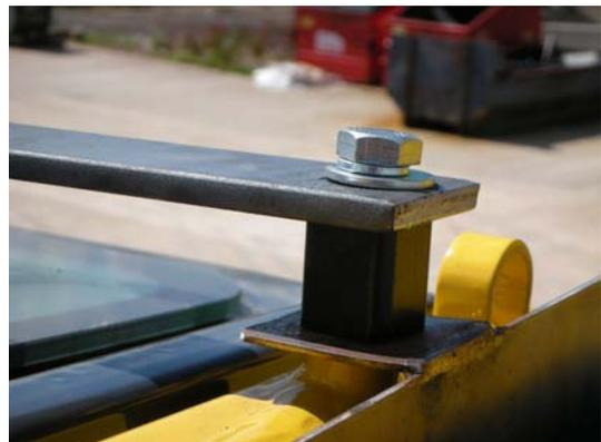
Remove the two plastic bungs from the threaded bosses at the bottom of the front screen and fit the front lower locking bar as shown in **fig 3**.
