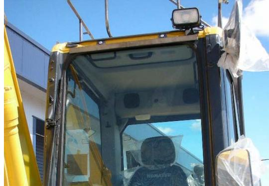
Remove the working light from the front of the machine as shown in **fig 1**, fit the hanging channel with 2 x M10 x 20 mm lg sets and spring washers, then refit the light onto the light stem with 1 x m10 x 25 mm lg set, washer and nyloc nut as shown in **fig 2**.
