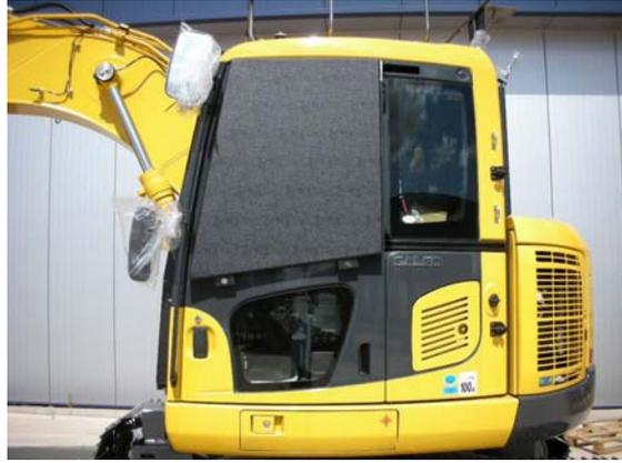
Fit the door hanging rail ensuring it is flush with the top and back edge of the door, as shown in [fig 11](#), drill the right hand side hole of the channel first, then secure with the pop-rivets supplied, work along from right to left drilling and securing each one in turn, the rail will then follow the contour of the door profile. Hang the door guard as shown in [fig 12](#) drill and fix as before.
