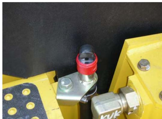
On the boom side **fig 6** loosen m12 bolt and move the bracket out to avoid it from fouling on the window guard then tighten back up (the guard will require trimming if it still catches).
